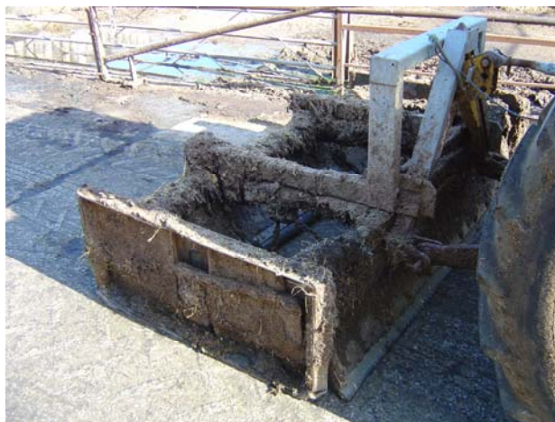
Fig 3: A box scraper will scrape cleanly, especially along kerbs, but will also save labour time making it an extremely cost effective
