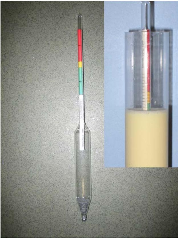
**Fig 4: A floating hydrometer that is specifically calibrated is useful for measuring colostrum quality**
